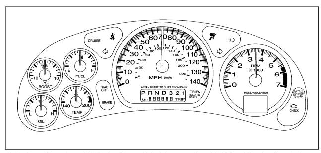
Uplevel 3800 Supercharged V6 Engine Cluster: United States version with ABS and Traction Control shown, Canada similar
